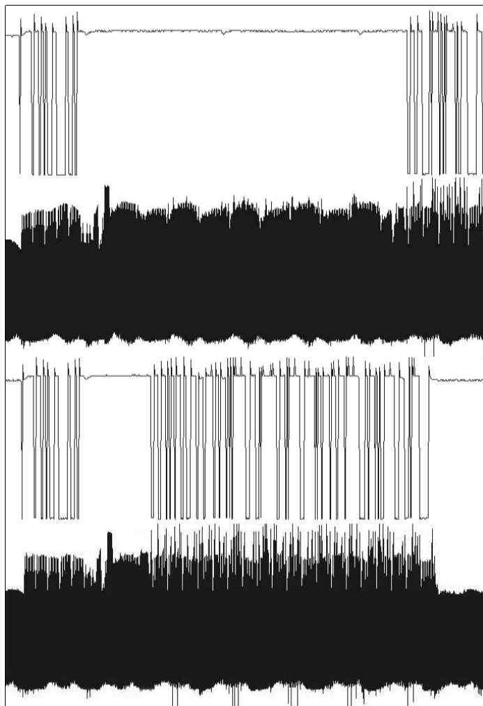
Fig. 3. The acquisitions from top to bottom: The I/O trace of a normal AES execution and its current consumption, where the rounds can be seen. Followed by the I/O trace of an AES execution where the number of rounds have been reduced to one and the current consumption showing the reduction in the number of rounds.
